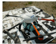
5 kg payload delivery drone prototype
